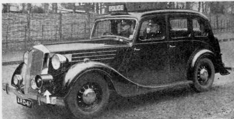
LOUD HAILER ON THE ROAD. A Hampshire Constabulary police car, fitted with an Ardente re-entrant horn loudspeaker of a type similar to that used as a marine "loud hailer" during the war. The speaker is stated to have a reliable range of 20-25 yards for talking to fast-moving cars; for pedestrian control the range is over 100 yards.
